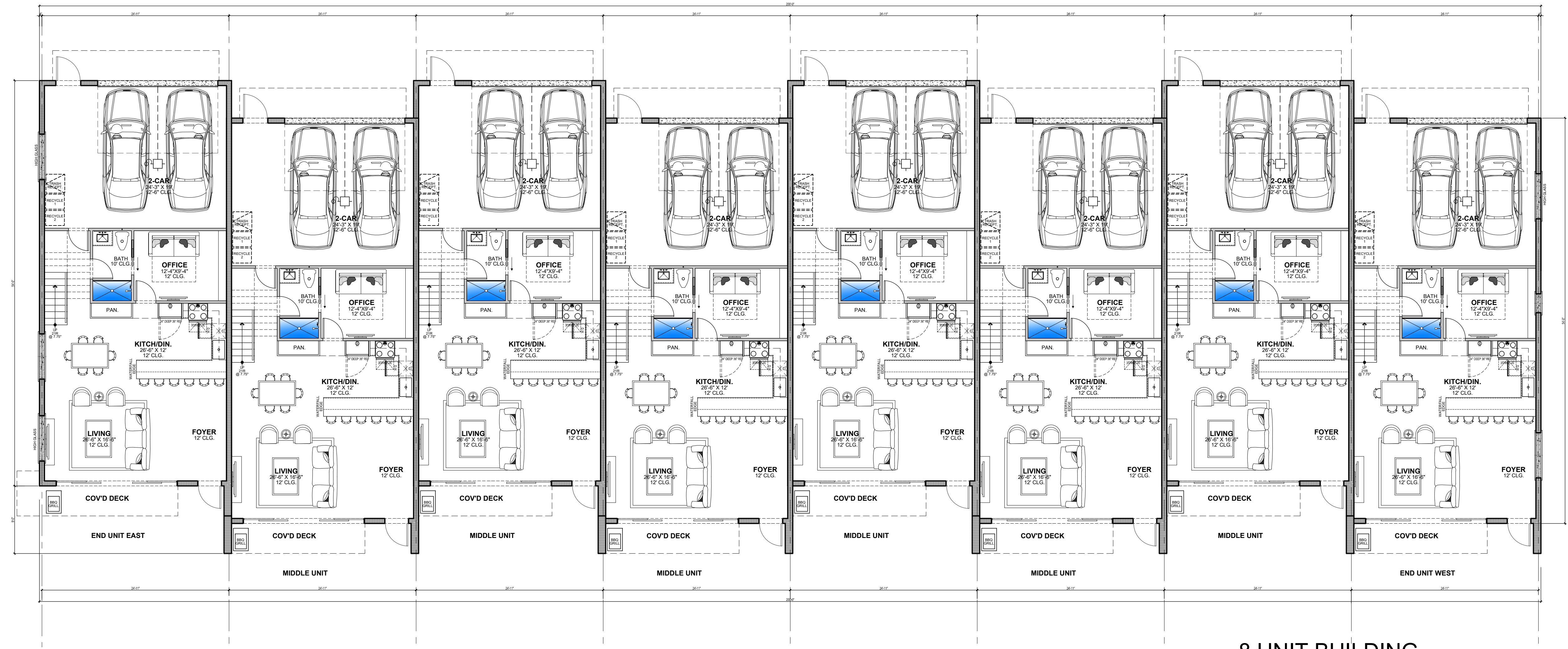
8 UNIT BUILDING FIRST LEVEL OVERALL PLAN SCALE: 1/8" = 1'-0"
